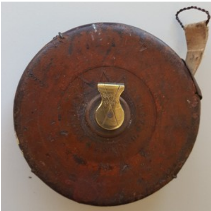
Abbey & Hockley 66ft fabric tape with leather case & brass rewriter
